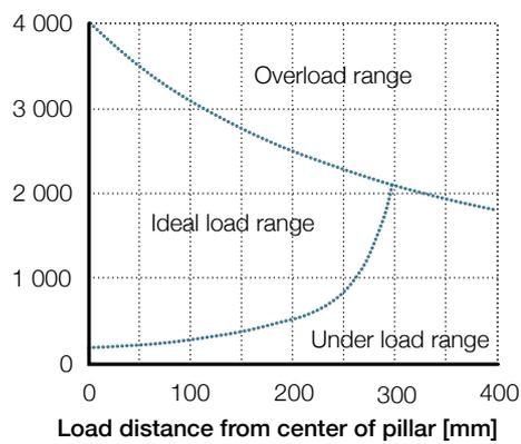
Bending load diagram 3-section
